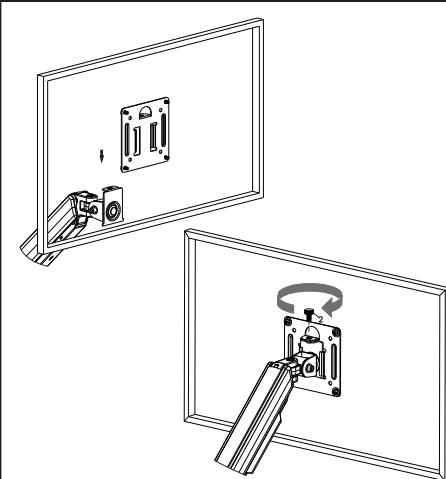
3. When the monitor is tilted automatically, tighten the set screw with wrench 3
