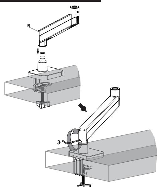
1. Insert the lower arm into the base, and fix the fastening screws on the base of the lower arm with a wrench 3.
