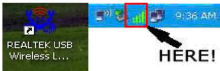
Left-click the icon will launch wireless network configuration utility, and you can right-click the icon to show the quick menu of configuration utility. This icon also uses different color to show the status of wireless connection:
