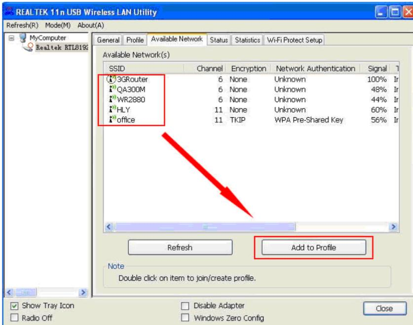
If the wireless access point you wish to connect does not appear here, you can click 'Refresh' button to scan for wireless access points again; if the wireless access point you're looking for still not appear, try to move the computer closer.
