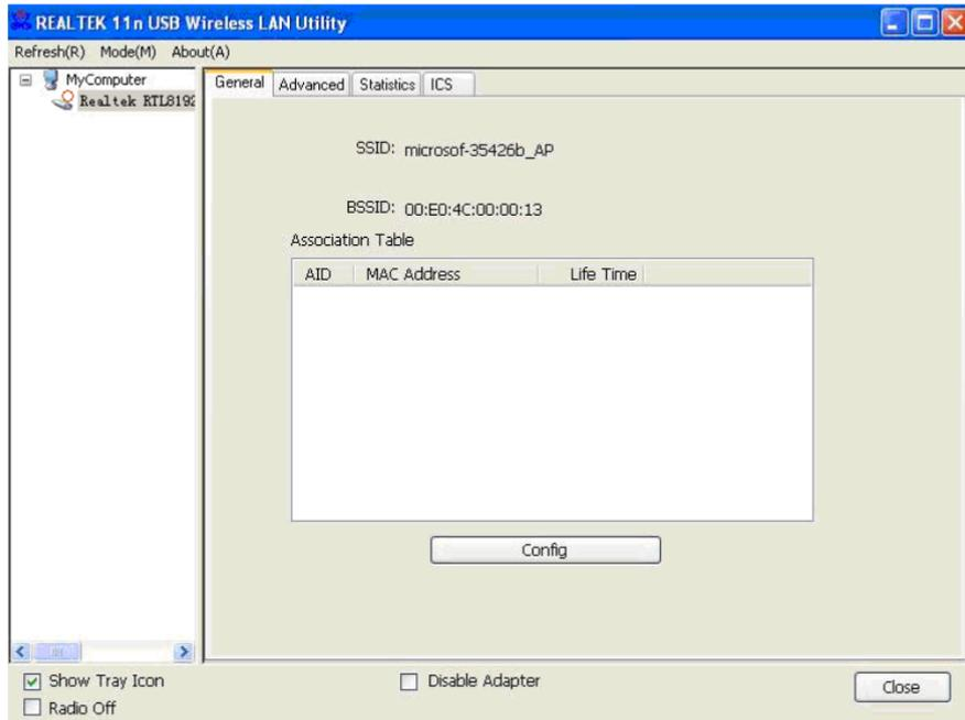
After mode switch is complete, you'll see general information of software AP, which shows AP's SSID and connected wireless clients.
