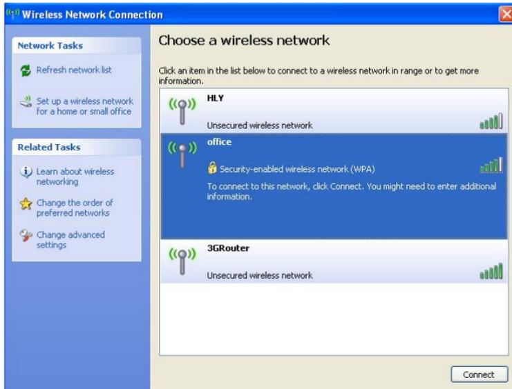
If the access point is protected by encryption, you have to input its security key or passphrase here. It must match the encryption setting on the access point. If the access point you selected does not use encryption, you'll not be prompted for security key or passphrase.
